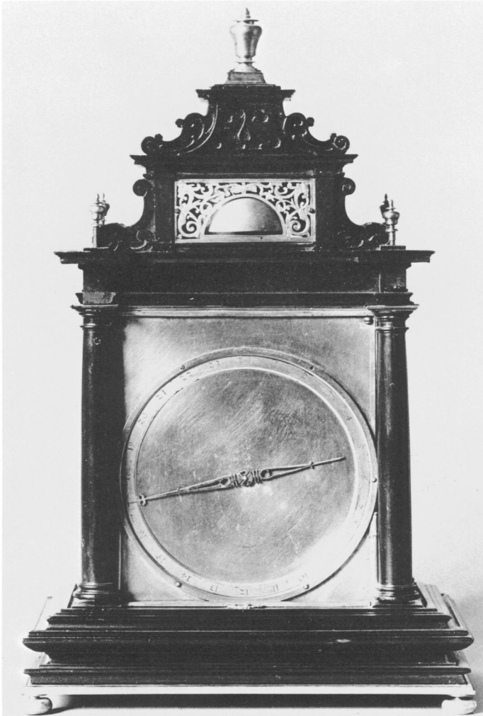
1. Experimental clock with a cross-beat escapement and with hour-striking and twelve-hour remontoire winding mechanisms, made by Jost Bürgi before 1600. H. 12 \frac{3}{8} in. (32.1 cm.). Kassel, Staatliches Landesmuseum, Astronomisch-Physikalisches Kabinett (photo: Staatliches Landesmuseum)
